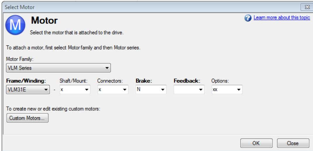
**Workbench setup, Custom Motor “create a motor file”** it is used for Kollmorgen brand motors not found in the Workbench motor data base or it can be used for 3<sup>rd</sup> party motors file creation. \* **F1 for HELP**- \* **Definitions** for the parameters used in motor setup can be found in the help section (F1) of the Workbench. **“MOTOR”**.
