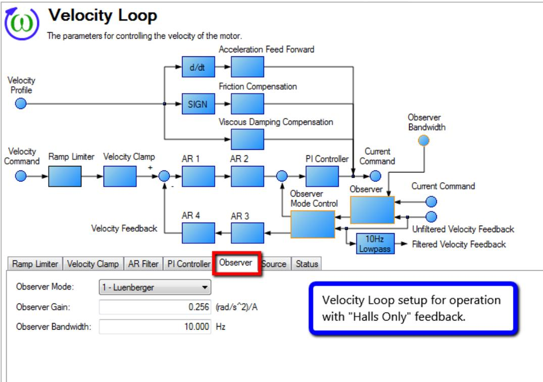
Velocity Loop setup for operation with "Halls Only" feedback.
